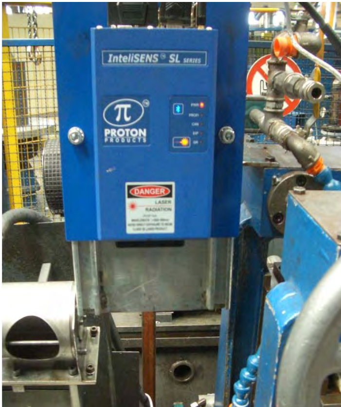
Cut to length control on continuous tube welding line.
