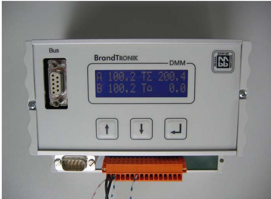
Processor based, modular structured, hybrid multi-channel measuring system for transducers in strain-gage-technics.
